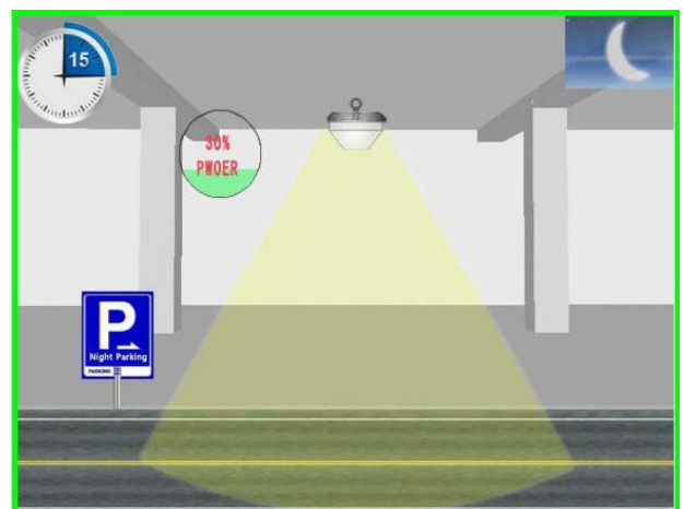
Mode 4: After a period people left (the period can be set), lighting brightness recover to 30%
