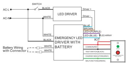
1.DO NOT MATE CONNECTOR UNTIL INSTALLATION IS COMPLETE AND AC POWER IS SUPPLIED. 2. TEST ACCESSORY LEADS-OBSERVE PROPER POLARITY WIRING.
