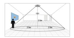
When the person is in the sensing area, the light will stay on until the person leaves;
